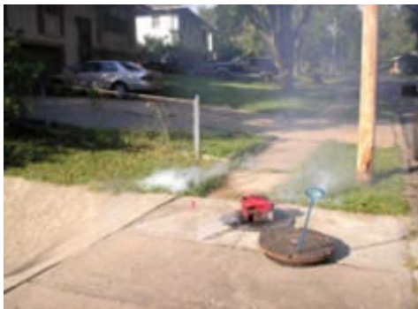
High-capacity blowers are used to pump smoke into a manhole (left photo). In the right photo, smoke is pushed into the system and emerges from cracks in the sidewalk and at a downstream manhole.
