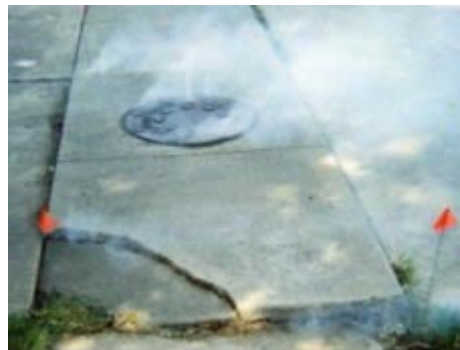
High-capacity blowers are used to pump smoke into a manhole (left photo). In the right photo, smoke is pushed into the system and emerges from cracks in the sidewalk and at a downstream manhole.
